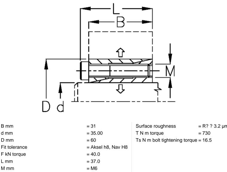
P N/mm2 surface pressure on shaft/hub = 95
